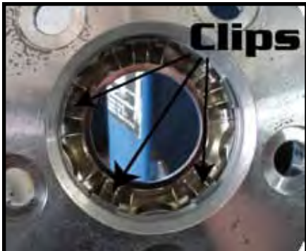
Clad wheel - inside - cone from this side with a standard taper cone and you hit the retaining clips, or hit the rear surface of the cladding
