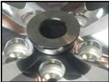
Clad wheel - outside - cone from this side and you are on the plastic, not the wheel
